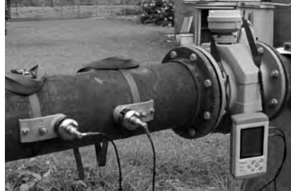
Prosonic Flow 92 used for the measurement consistency check of an electromagnetic flowmeter (see page 27)
