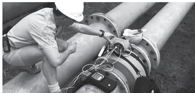
On-site functional check of a flowmeter using FieldCheck®
