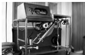
Mobile flow rig for on-site calibration
