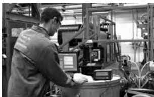
On-site calibration of temperature instruments
